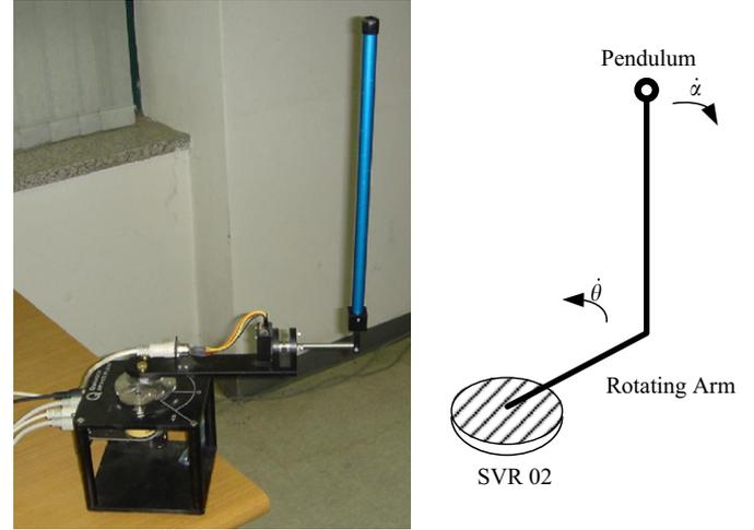
Fig. 1. Rotary inverted pendulum system.
