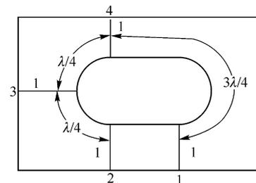
Fig. 2 Racetrack microstrip hybrid ring on rectangular substrate
