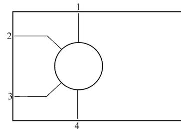
Fig. 1 Standard microstrip hybrid ring on rectangular substrate
