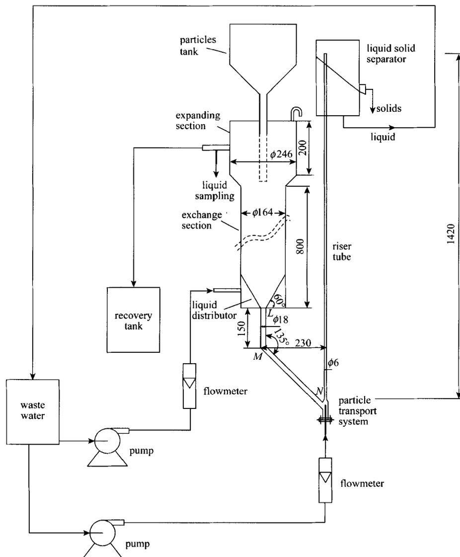
Figure 1 The schematic diagram of the pilot system
