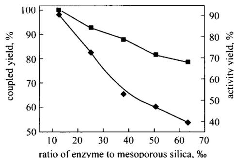
**Figure 2** Effect of mass ratio of enzyme to mesoporous silica on the coupled yield and activity yield of assembled PA
