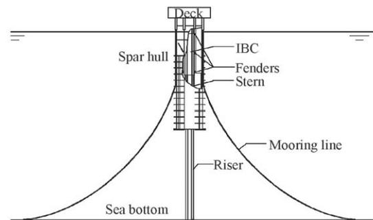
Fig.2 The coupled system (with distorted scale of water depth)
