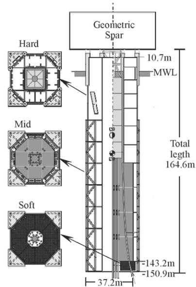
Fig.1 Configuration of the geometric spar
