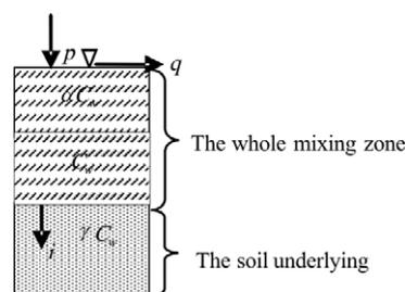
Fig.1 Sketch of simple two-layer model
