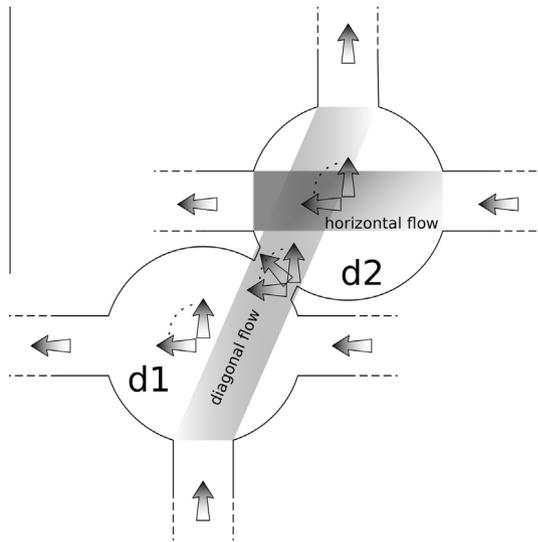
**Fig. 2.** The magnetization in the leads is fixed and oriented along  $180^\circ$  for horizontal leads and along  $90^\circ$  for vertical leads. The disks can be switched between the two states by either applying a horizontal or a diagonal current. At the constriction the resulting magnetization is a superposition of the magnetizations in  $d1$  and  $d2$  and, therefore, the magnetization at the constriction is switched in multiples of  $45^\circ$  between  $90^\circ$  and  $180^\circ$ .
