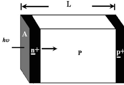
Fig. 1. Cross section of the  $n^+pp^+$  HgCdTe photodiode.
