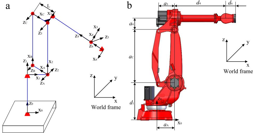
Fig. 1. DHm parameterization of the robot with kinematic parallelogram. (a) Kinematic modeling. (b) Kinematic parameters.
