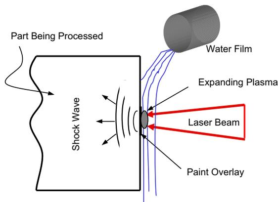
Fig. 1. Schematic of laser shock peening (LSP).
