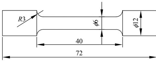
Fig.1 Tensile specimen of CuW70 alloys
