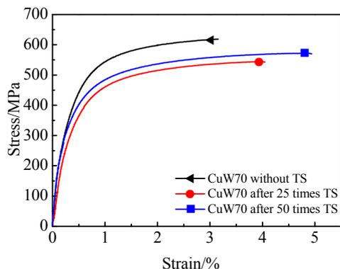
Fig.2 Stress-strain curves of CuW70 alloys under tensile load
