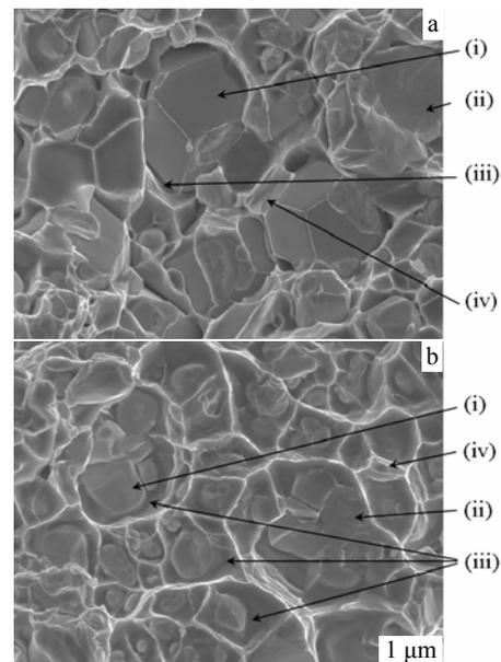
Fig.3 Fracture surface of CuW70 alloys under tensile load: (a) fracture surface morphology without thermal shock, (b) fracture surface morphology after 50 times thermal shock; (i) intercrystalline fracture, (ii) transgranular cleavage, (iii) dimple, (iv) tearing
