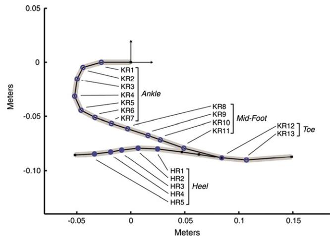
**Fig. 2.** The prosthetic foot model included 22 rigid segments connected in series by 13 keel (KR1–KR13, ●) and 5 heel (HR1–HR5, ●) revolute joints. Black squares indicate segment endpoints where rotational degrees-of-freedom are not present.
