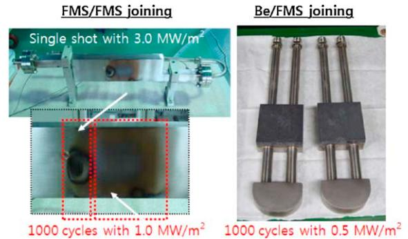
Fig. 4. Fabrication technology development: FMS/FMS and Be/FMS joining.
