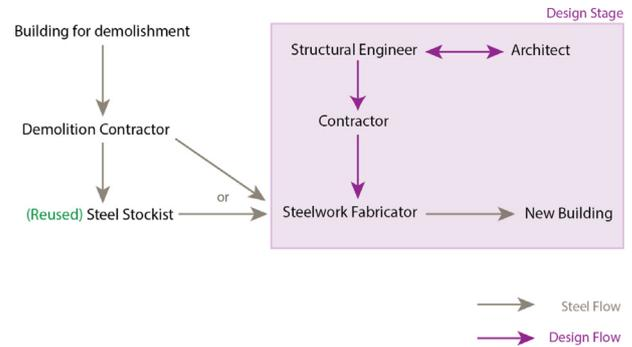
Fig. 1. Mapping steel reuse flows for relocated reuse.
