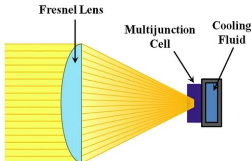
Fig. 1. Component Drawing of the Linear Concentrating Photovoltaic System.
