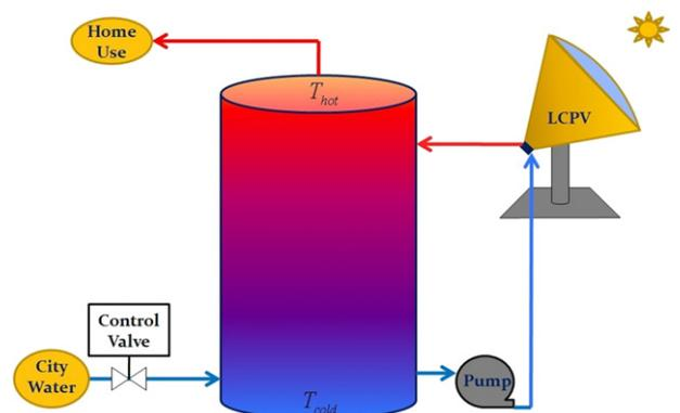
Fig. 2. LCPV System with Flow Diagram.
