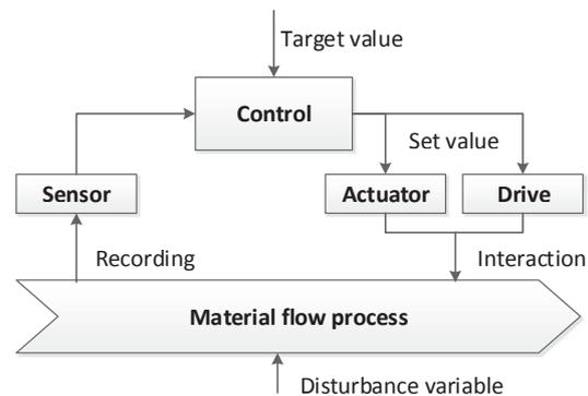
Fig. 2. Principle of automated material flow systems
