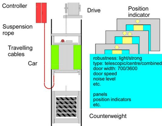
Fig. 2. Schindler elevator components.
