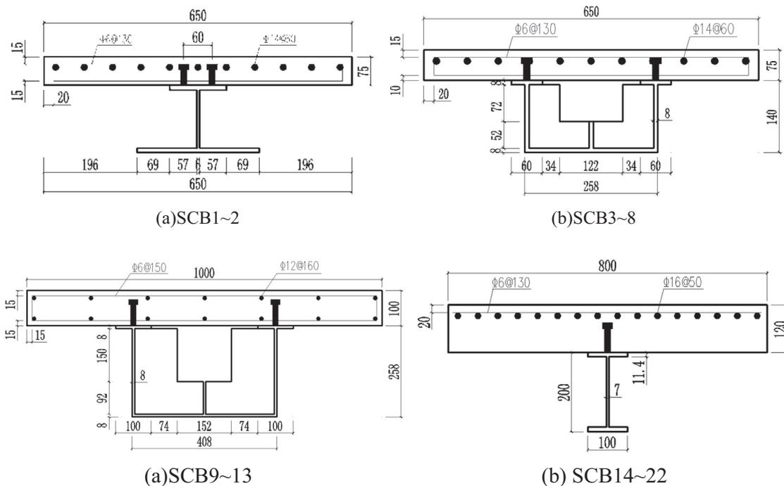
Fig. 1. Cross section details of the girder.
