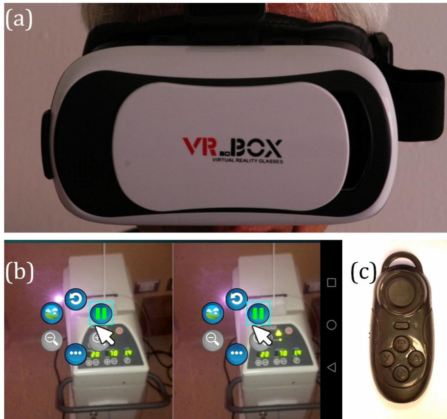
**Fig. 1.** Augmented Reality device. (a) VR BOX II virtual reality glasses; (b) screenshot of the smartphone display with the image captured by the rear camera and the superposed popup menu of the SuperVision app, and (c) the handheld Bluetooth controller.
