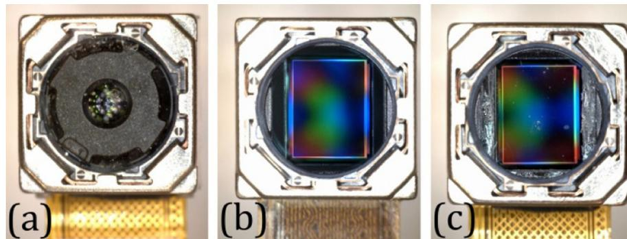
**Fig. 2.** The Sunny P13N05B rear camera module (a) with the objective lens in place, (b) the objective was unscrewed, the Infrared Cut Filter and, beyond, the CMOS image sensor, are visible and, (c) the IR filter was removed. Some damaged areas of the sensor are visible.
