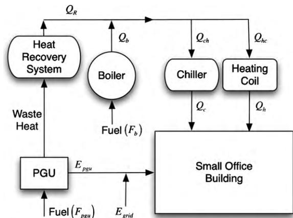
Fig. 1. Schematic of a CCHP system.
