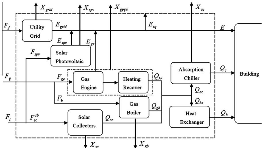
Fig. 1. The energy and emission flow chart of the solar BCHP system. The thin solid line and thick solid line represent the energy flow and emission flow respectively, and the equipments inside the dotted line are a package unit.
