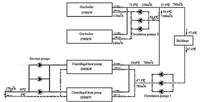
Fig. 1. Flow chart of the hybrid heating system.
