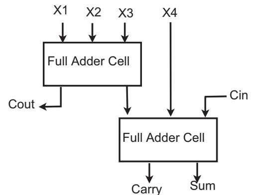
Fig. 3. Conventional 4-2 compressor structure.
