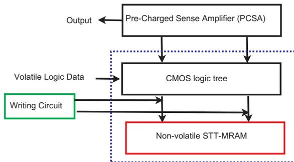
Fig. 2. Structure of a MTJ based circuit.
