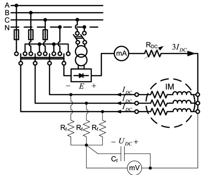
Fig. 1. Schematic display of the system for continuous measurement of stator winding resistance.
