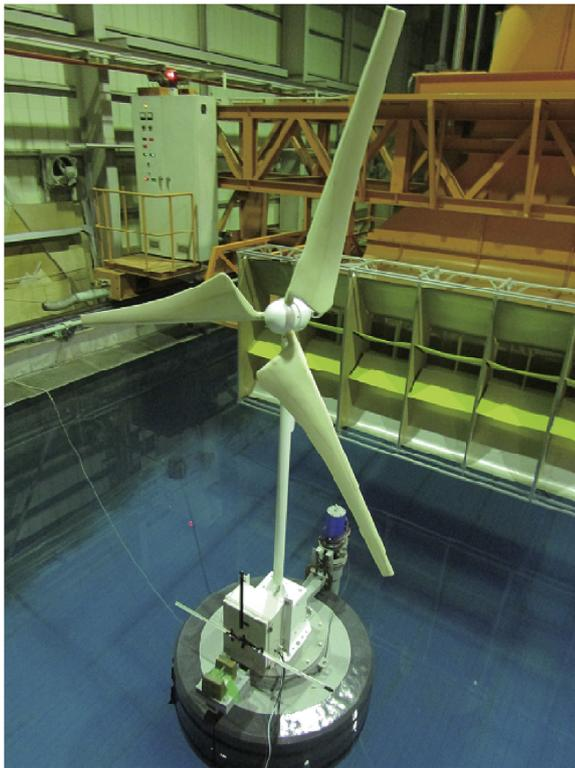
Fig. 1. Photo of the floating offshore wind turbine.
