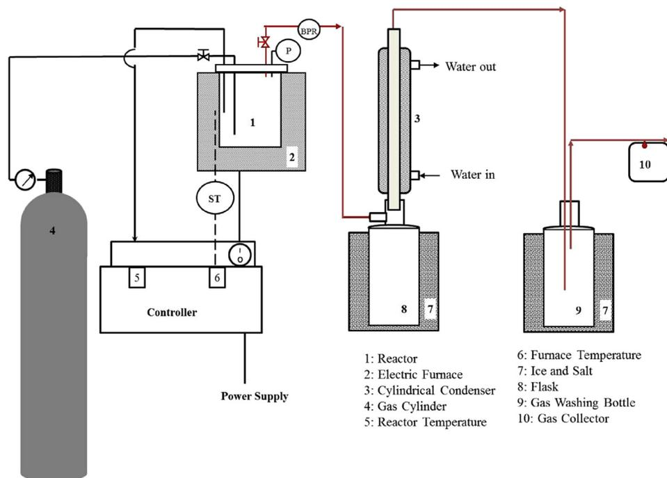
Fig. 1. Schematic of pyrolysis experimental set-up.
