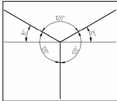
Fig 1 Isometric axes in image plane [2]
