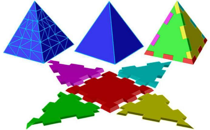
Fig. 2. Overview of the production system for planar structures bevel joints.
