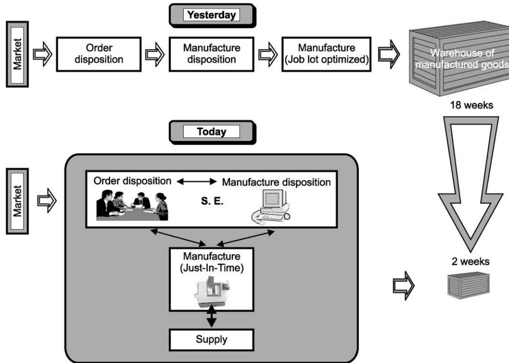
Fig. 1. Principle of work of modern production management.
