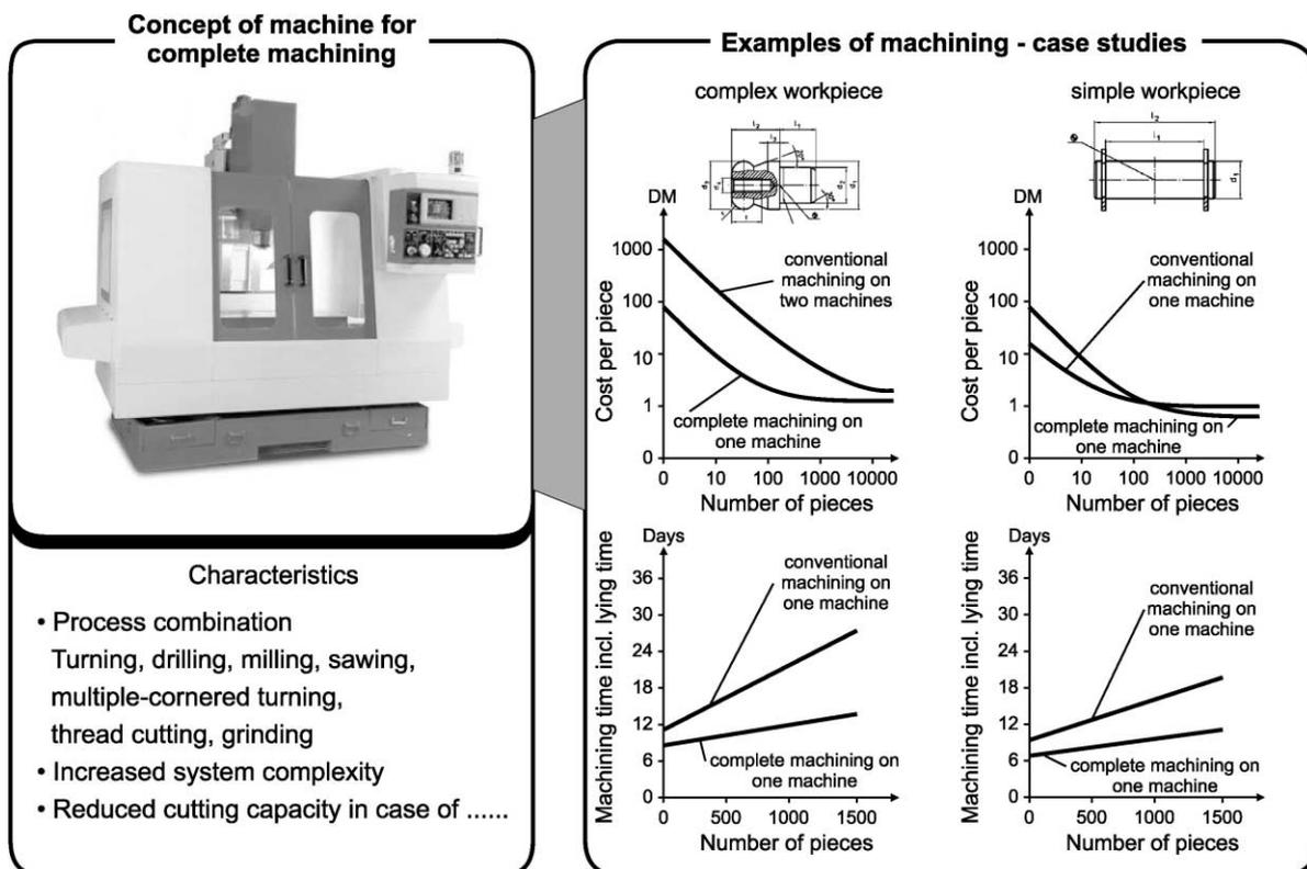
Fig. 2. Comparison of conventional method of machining of standard components with the method of complete machining.
