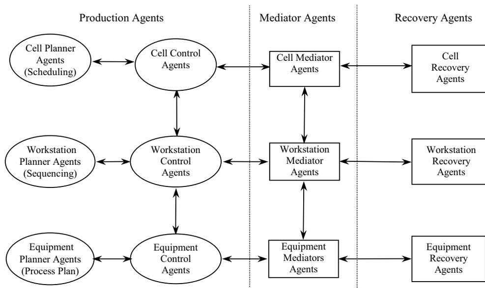
Fig. 1. Intelligent-agent-based hierarchical architecture having error recovery agents.
