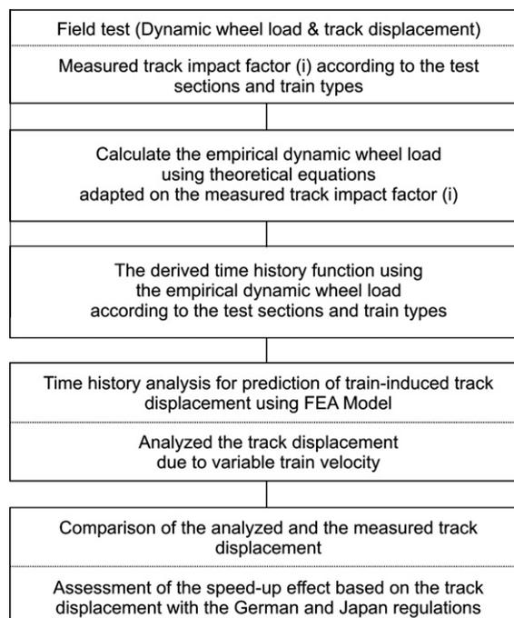
Fig. 1. Procedure of prediction of train-induced track displacement.
