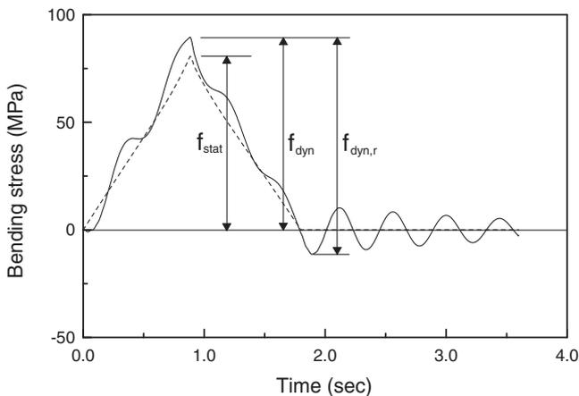
Fig. 1. Example of bending stress time history at center of simple span bridge.
