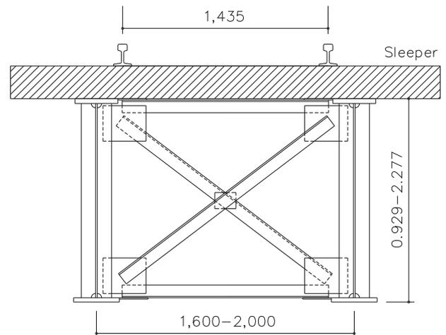
Fig. 2. Typical cross-section of a study bridge (unit: mm).
