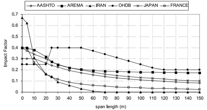
Fig. 1. Impact factor based on various codes.
