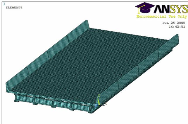
Fig. 2. A finite element model for Bridge 2.
