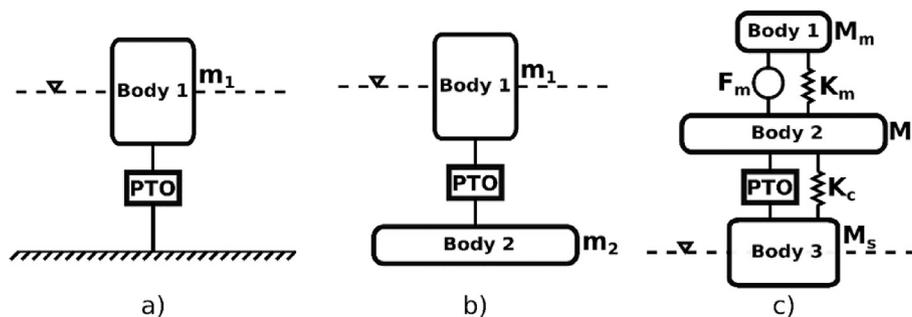
Fig. 1. WEC architectures of growing complexity in the point absorber class. a) Single-body; b) Self-Reacting Point Absorber; c) Korde's WEC [9].
