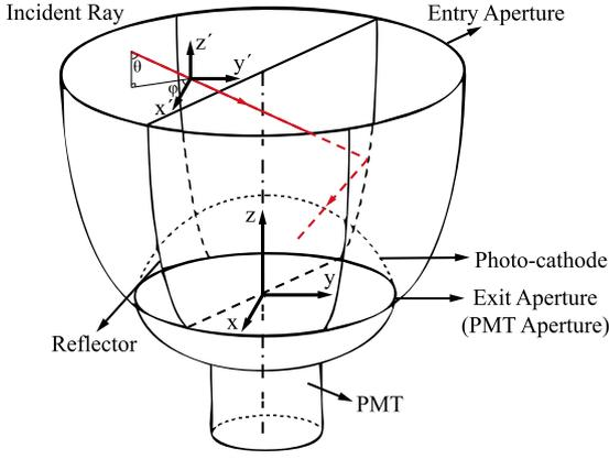
Fig. 1. Illustration of a PMT with a concentrator. The incident angle,  $\theta$ , is the angle between the incident ray (red line) and the symmetry axis ( $z$  axis). The azimuth angle,  $\phi$ , is the angle between the  $x$ -axis and the projection of incident ray on the  $x$ - $y$  plane. The  $x$ -axis is arbitrary unless specified. The entry aperture, exit aperture (PMT aperture) are parallel to the  $x$ - $y$  plane. More details are explained in the text. (Color online)
