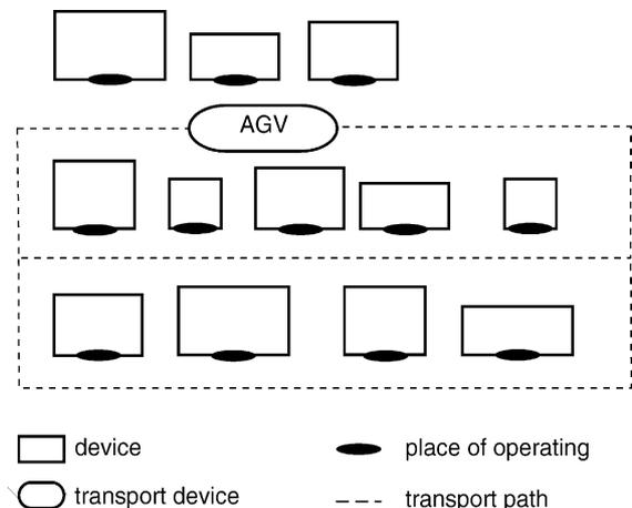
Fig. 1. Layout of devices fed by AGVs in multiple rows.
