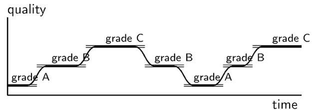
Fig. 1. A product grade slate A–B–C–B–A with on-spec-ranges.
