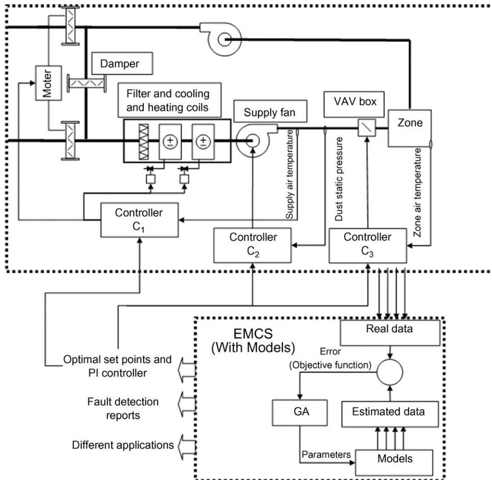
Fig. 1. Typical HVAC system and EMCS along with the proposed models.
