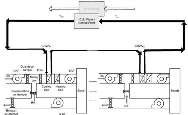
Fig. 1. Schematic diagram of a typical HVAC system for cooling purpose.
