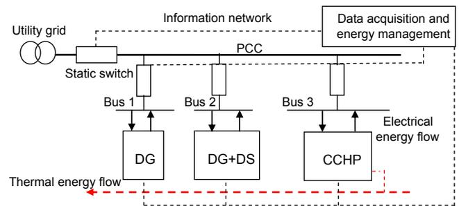
Fig. 1. Micro-grid, distributed energy generation and storage. Adapted from Lasseter (2002)
