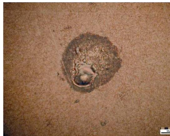
Fig. 3: View of a crater produced at the surface by the spark. Melted material can be seen [2].
