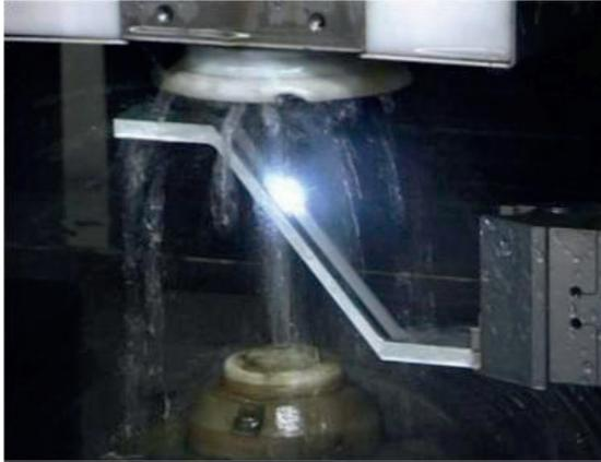
Fig. 1: Wire EDM production of a complex part.
