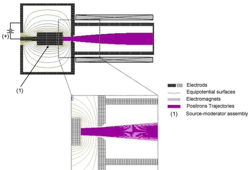
Fig. 2. Simulation of the positron trajectories in the PG acceleration region.
