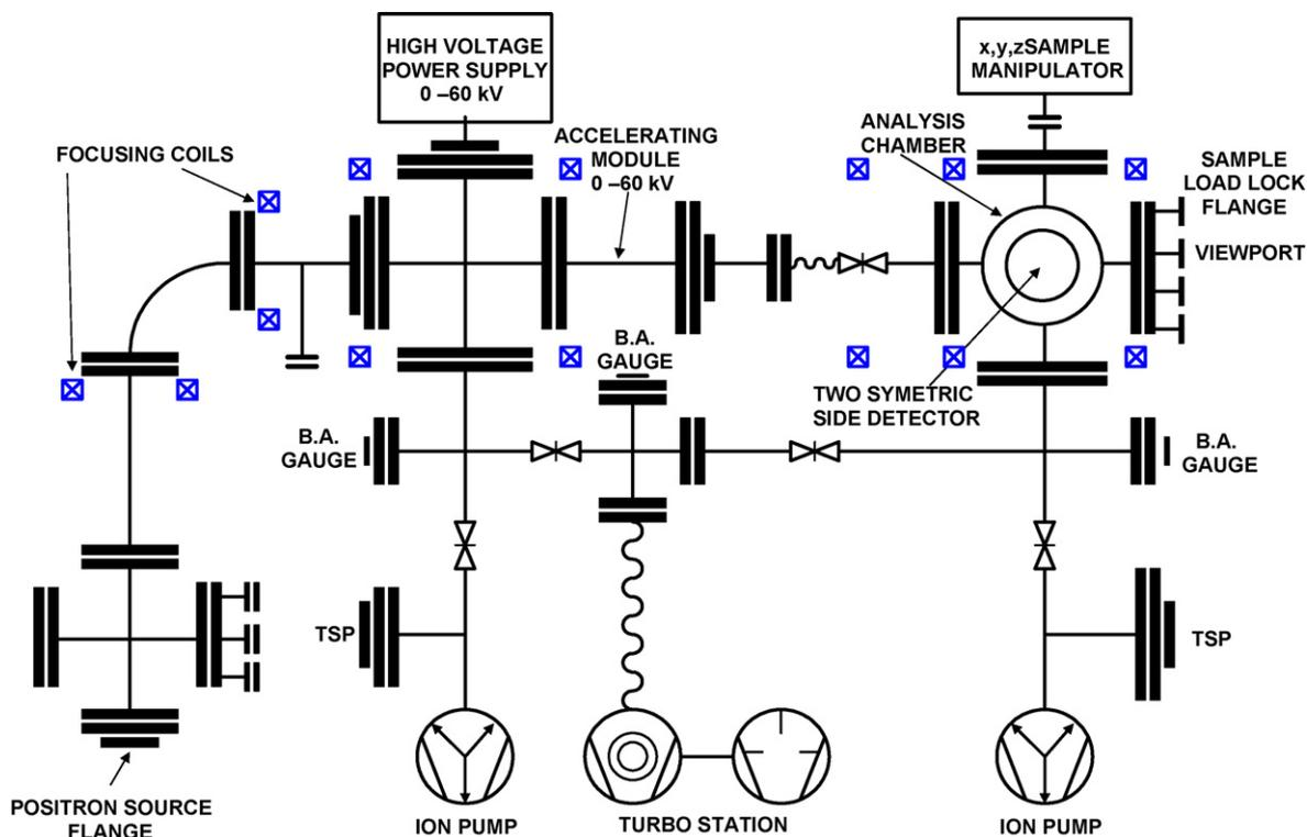
Fig. 1. The schematic of the positron gun.
