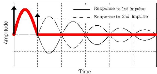
Fig. 1. Basic idea of IST; the responses (thin solid and dashed lines) caused by two impulses (vertical arrows) are superposed to result in nonvibratory response (thick line).
