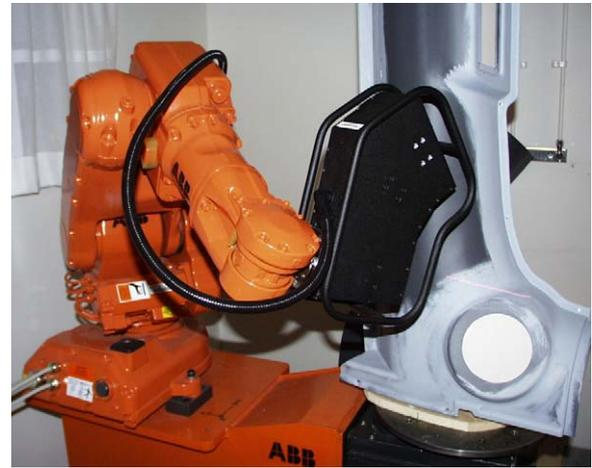
Fig. 2. The robot scanning system comprises an industrial robot, a turn-table and a laser profile scanner.
