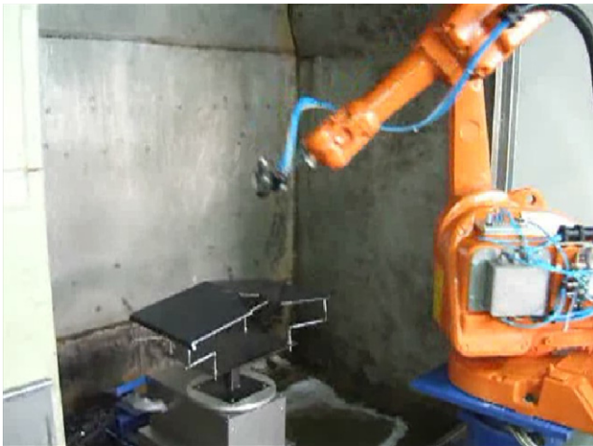
Fig. 1. Paint robot with hoses. Hoses may be tangled on the robot arm.
