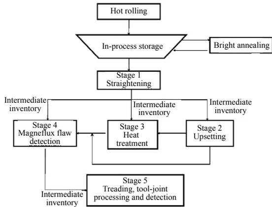
Figure 1. Production process schematic for seamless steel tube
