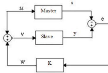
Fig. 2. Controlled master-slave system
