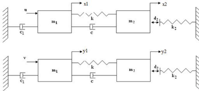
Fig. 3. Analogical spring-dumper-mass master and slave systems.
