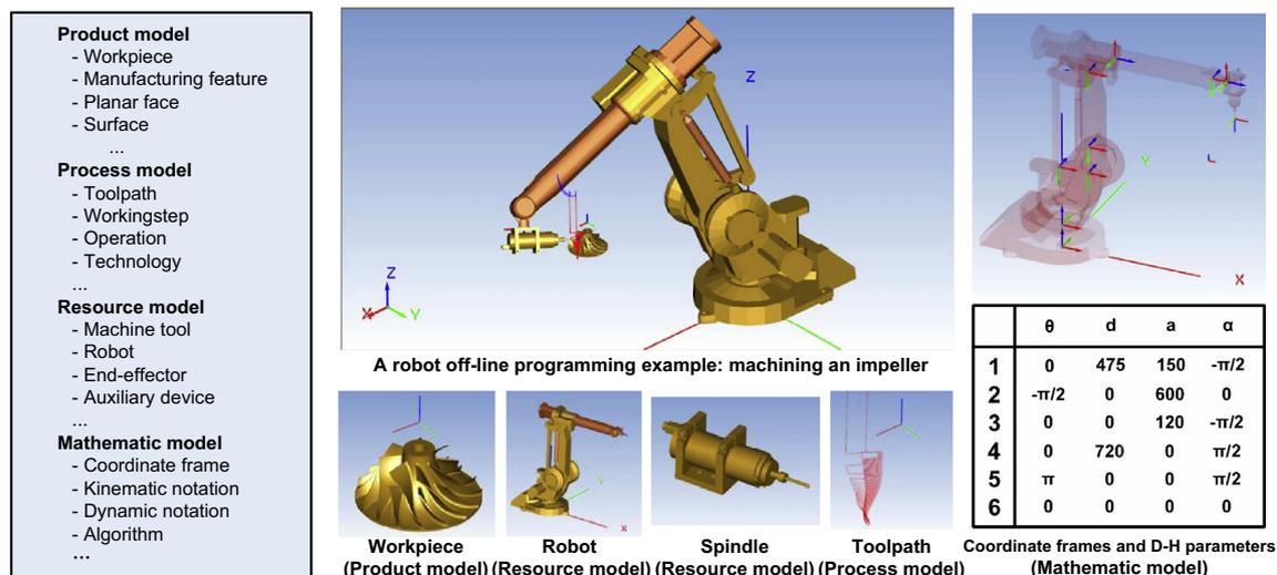
Fig. 1. Model categorizations of the IRDM and an instance of robot off-line programming.
