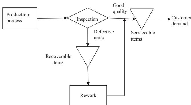
Fig. 1. The production system with rework.
